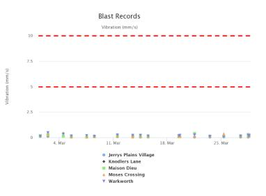
Figure 82: Ground Vibration Blast Monitoring Results – February 2019
